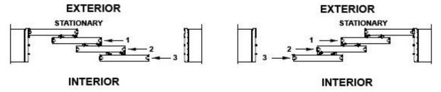
•Units with stationary panels on the interior most track will need to be assembled in a reverse order than described here. Installation is the same, but the first panel to be installed is on the interior most track working outward with panels.
