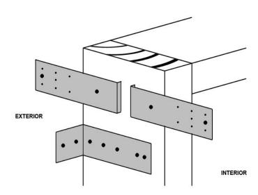
protruding towards it. Approximately 3  $\frac{1}{2}$ " of the flat end of the clip should be sticking out from the exterior of the jamb. Fasten using a #10 x 1" pan head screw. When installed properly the end with the small leg will be slightly bent to stop the clip from spinning.
