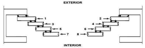
•Units with a pocket only on one side are numbered in a similar fashion. These units will only have one panel per track and will be numbered starting with "1" counting inward from the exterior. This numbering is the same regardless of the location of the pocket on either the left or right side.
