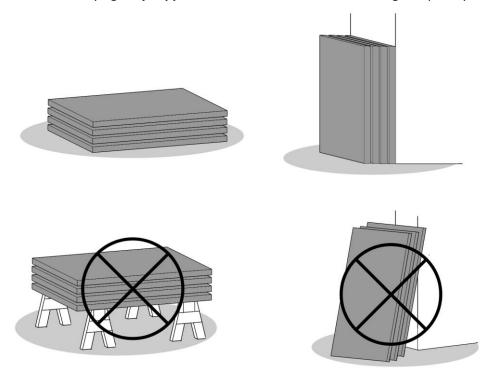
**WARNING-** DO NOT store panels in a standing/leaning position, or laying flat on saw bucks or blocks of any fashion. Improper storage can diminish the performance and life of the units.
