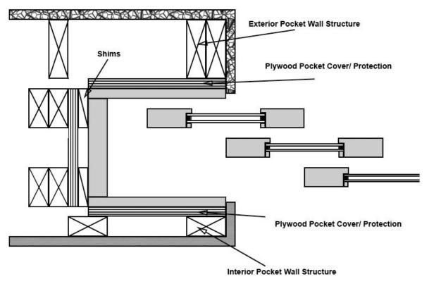
•The wall next to the pocket must be plum, level, and straight within a 1/8" tolerance. When fastening framing or trim near the pocket opening use a string line to keep the pocket opening straight. A bow in the pocket opening may contact and damage panels, prevent the unit from sealing, or cause improper operation.
