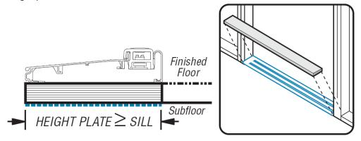
•A completed sill opening will be a single smooth, flat, level plane on which the jamb will rest.
